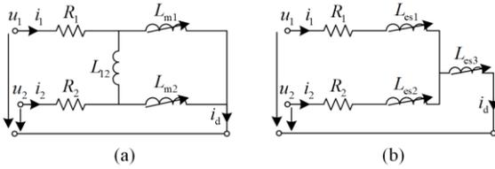
Fig. 3. Equivalent inductance model. (a) Model with delta structure. (b) Model with wye structure.
