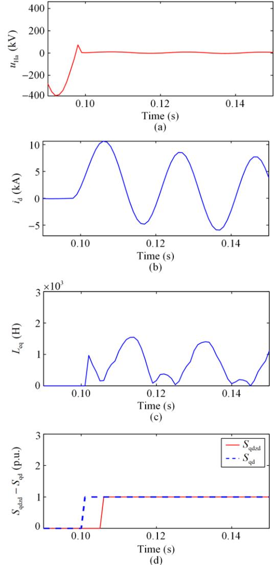
Fig. 20. Test results of phase-to-ground fault in HV lead wire. (a) HV winding voltage. (b) Differential current. (c) Equivalent inductance  $L_{eq}$ . (d) Mark signals.
