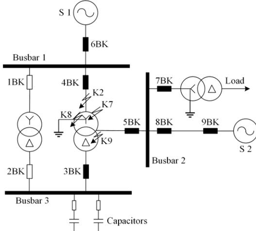
Fig. B1. Physical dynamic model system.
