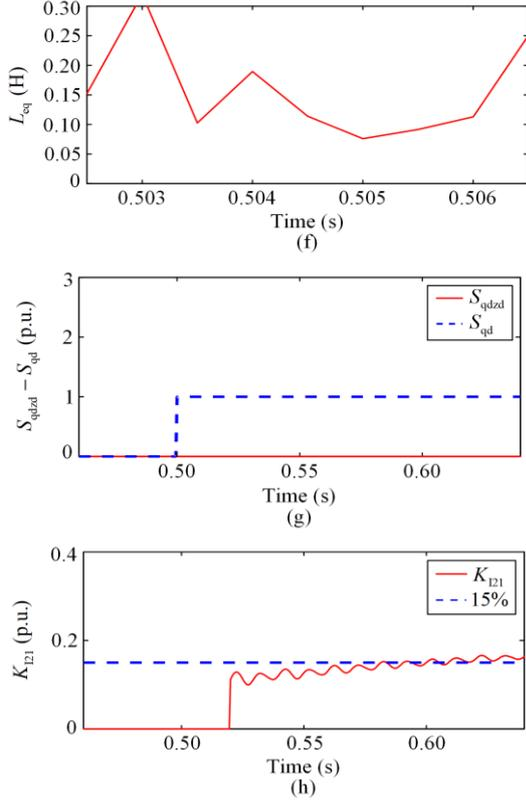
Fig. 22. Test results for inrush current in 500 kV autotransformer using transformer protection data. (a) Voltages of HV, common, and tertiary winding. (b) Local waveforms of HV, common, and tertiary winding voltages. (c) Differential current  $i_d$ . (d) Local waveform of  $i_d$ . (e) Equivalent inductance  $L_{eq}$ . (f) Local waveform of  $L_{eq}$ . (g) Mark signals. (h)  $K_{121}$  of  $i_d$ .
