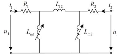
Fig. 1.  $\Pi$  equivalent model of single-phase two-winding transformer.
