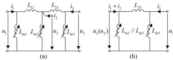
Fig. 12. Dual equivalent model of single-phase three-winding autotransformer. (a) Original model. (b) Transformed model.
