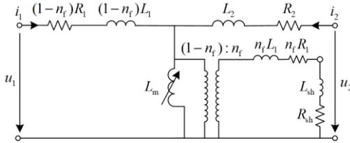
Fig. 9. Equivalent circuit of faulty transformer.
