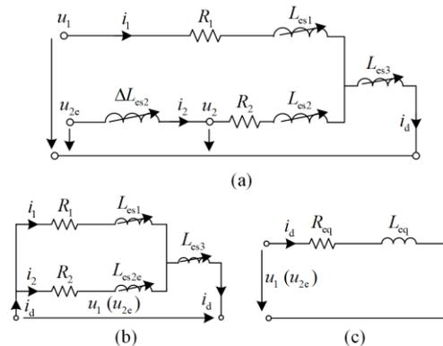
Fig. 6. Equivalent inductance model for Case 2. (a) Original model. (b) Transformed model. (c) Final equivalent model.
