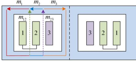
Fig. 11. Layout of single-phase three-winding autotransformer.
