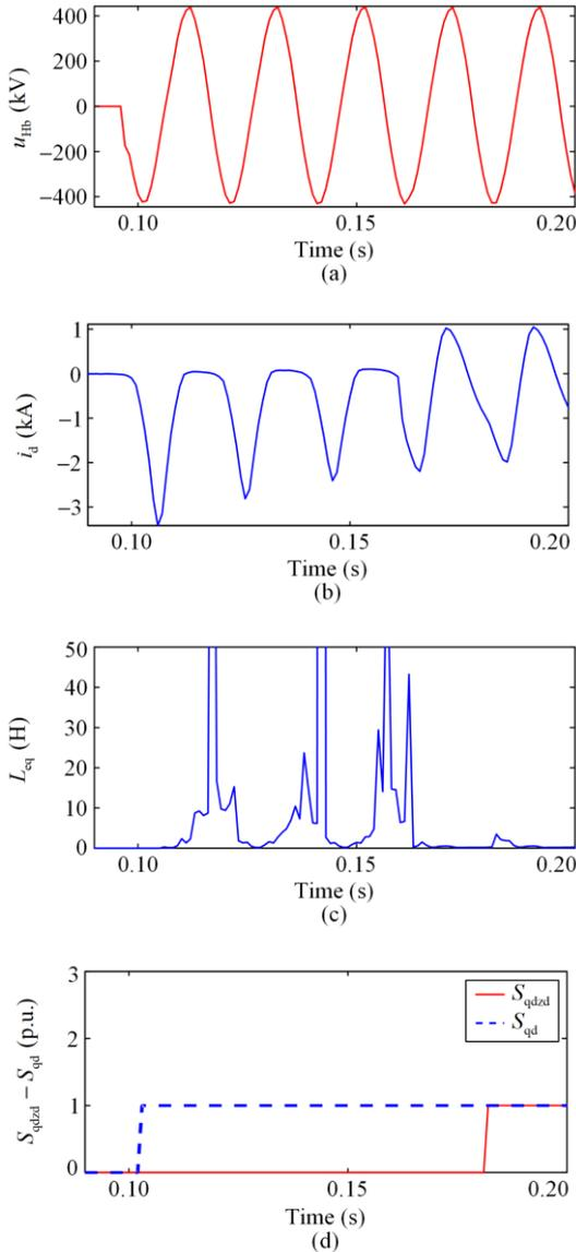
Fig. 21. Test results of inrush current with 2% turn-to-turn fault. (a) HV winding voltage. (b) Differential current. (c) Equivalent inductance  $L_{eq}$ . (d) Mark signals.
