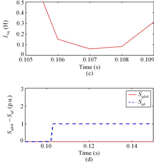
Fig. 18. Test results of inrush current. (a) HV winding voltage. (b) Differential current. (c) Equivalent inductance  $L_{eq}$ . (d) Mark signals.
