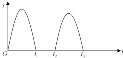
Fig. 4. Waveform of transformer inrush current.
