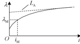
Fig. A1. Core saturation characteristics used in PSCAD simulations.
