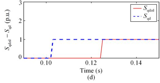
Fig. 19. Test results of 2% turn-to-turn fault in series winding. (a) HV winding voltage. (b) Differential current. (c) Equivalent inductance  $L_{eq}$ . (d) Mark signals.
