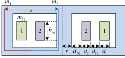
Fig. 2. Layout of single-phase two-winding transformer.
