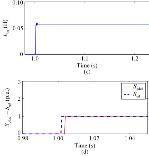
Fig. 16. Results of turn-to-ground fault simulation. (a) HV winding voltage. (b) Differential current. (c) Equivalent inductance  $L_{eq}$ . (d) Mark signals.
