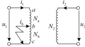
Fig. 8. Transformer fault diagram.
