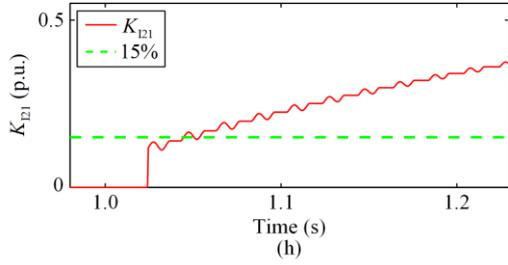
Fig. 14. Results of inrush current simulations. (a) Voltage of HV winding. (b) Local waveforms of HV and LV winding voltages. (c) Differential current  $i_d$ . (d) Local waveform of  $i_d$ . (e) Equivalent inductance  $L_{eq}$ . (f) Local waveform of  $L_{eq}$ . (g) Mark signals. (h)  $K_{121}$  of  $i_d$ .
